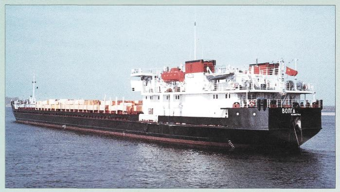
**Type of vessel** Sea-river going single deck twinscrew dry cargo motor vessel with double sides and double bottom, fitted with bowthruster.
