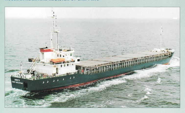
**Type of vessel** Sea-river going single deck singlescrew dry cargo motor vessel with double sides and double bottom, fitted with bowthruster.
